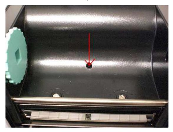
STEP 4: Separate the head from the module.
