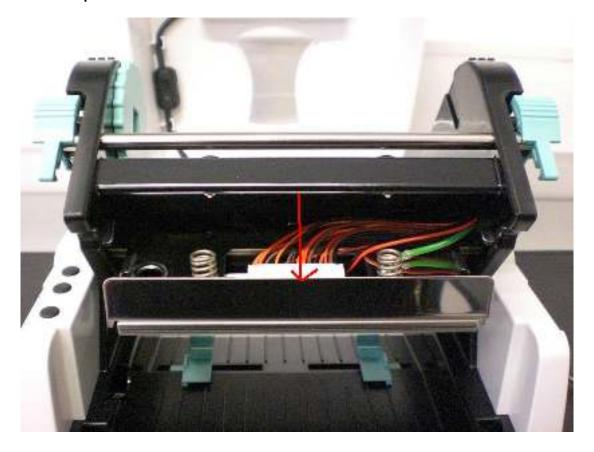
STEP 5: Separate the ribbon straightener from the head using the tabs.
