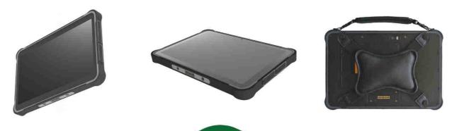
Intel N5100 8GB Ram, 256GB Storage Display 10.1" 1920 x 1200 WiFi, Bluetooth, 4G LTE Docking and Vehicle Cradle Ubuntu, open-source OS based on Debian
