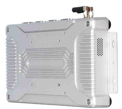
Ultra-Compact IIoT Gateway Edge Computing System based on High performance Intel's Technology
