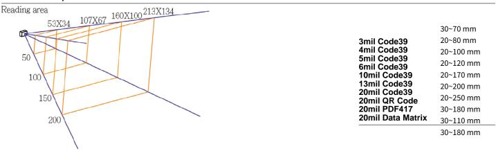
Note: the test is under ambient light 700  $\sim$  800 Lux.
